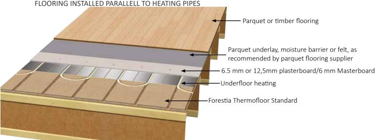
5 25 MM FORESTIA THERMOFLOOR EXTRA WITH 14 MM PARQUET OR TIMBER FLOORING INSTALLED PARALLELL TO HEATING PIPES
