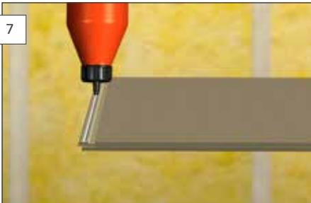
Cut and install the next panel. Remember to glue the short-end profile. We recommend PVAc glue or equivalent.
