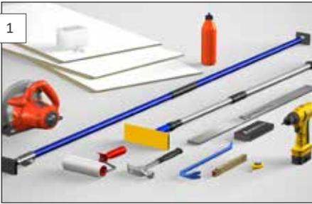
Have all the necessary equipment ready before installation starts. For ceiling surfaces longer than 8 m, extra clearance for expansion is required, min. 1.5 mm per metre of ceiling. Premium Ceiling panels are installed on min. 30-mm battens, or directly on existing ceiling panels. NB. The Forestia guide rails and tapping block are specially adapted to the profiles on Premium Ceiling panels.
