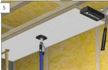
Use a ceiling support to hold up the panels during installation. The Forestia tapping block **must** be used to avoid damaging the profile when the panel is to be clicked into place. This tapping block is adapted to the panel's profile.
