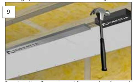
Forestia guide rails **must** be used from panel no. 2 onwards. It is essential that the panels are placed evenly against one another for optimum results. **Hold** the guide rail in place in the profile when using the tapping block to drive the panels close together. (Be careful that the guide rail doesn't fall down when in use).
